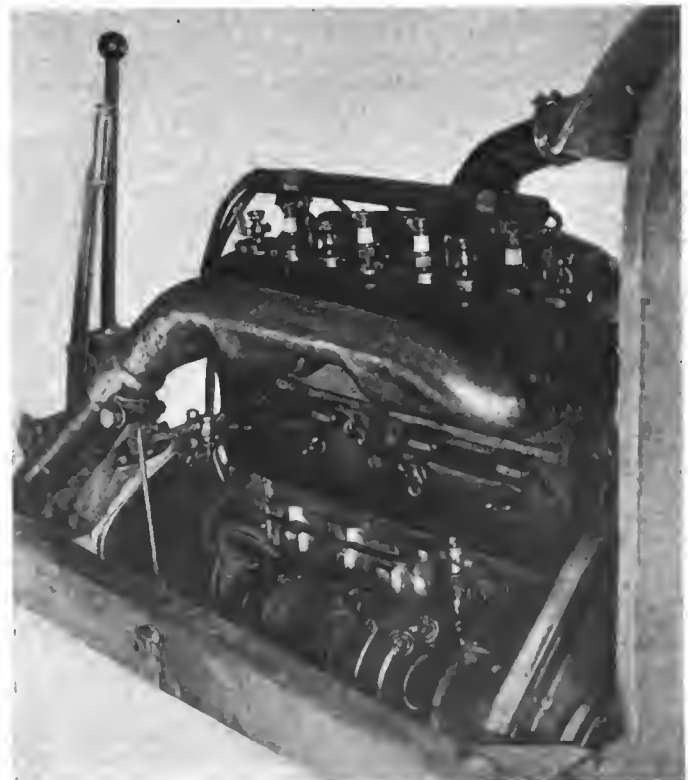
Kent power plant, showing magneto drive from generator
